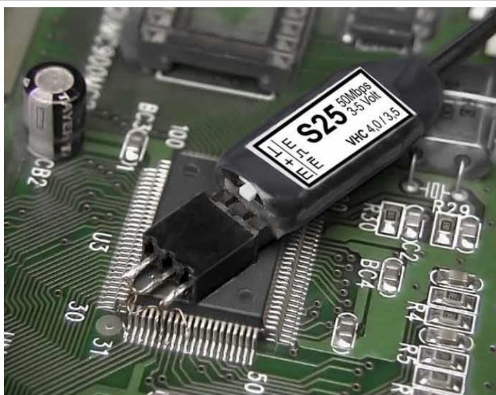
**Figure 2** S25 sensor integrated in the DUT
